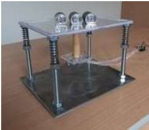
Figure 7 – Experimental model of a compaction table with lever fixturing of the vibration exciter under load
