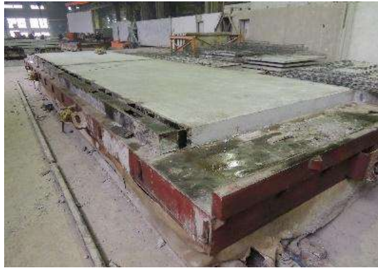
Figure 5 – The vibrating table with mounted exciters of oscillations
