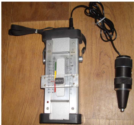
Figure 5 – The ISP-1 vibrometer for measuring the values of shock pulses (dB) at the test points of the experimental model of the compaction table
