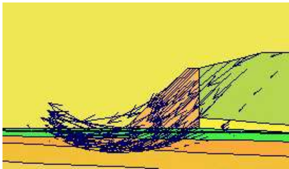
Figure 8 – Geometric model and results of SDM slope modeling
