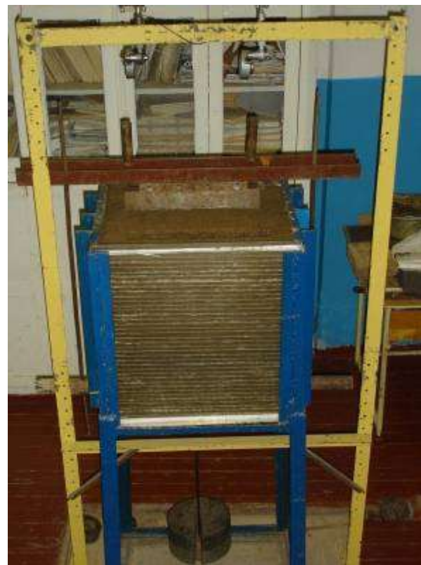
Figure 3 – The tray filled with soil paste for stamping tests during the experiment
