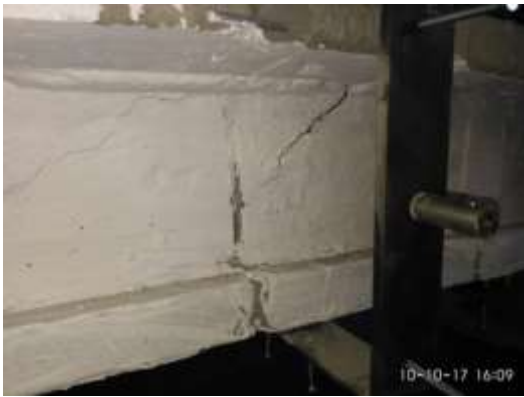
Figure 6 – Inclined crack from the top of the artificial normal crack in the beam
