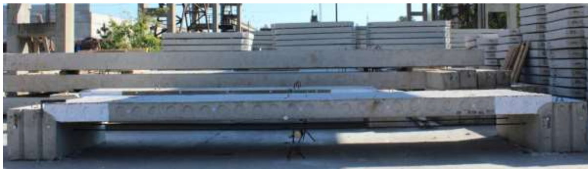
Figure 2 – Experimental design of the intercolumn plate on the test bench.
