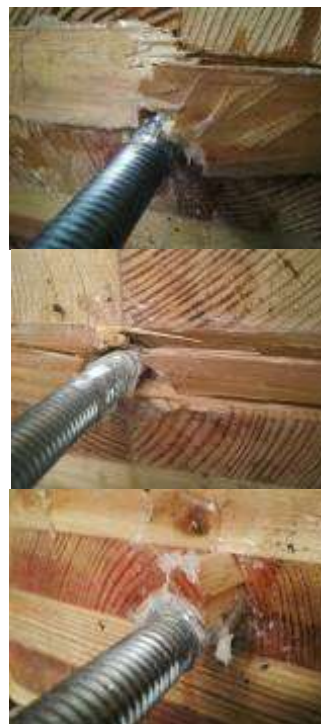
Figure 4 – Failure mode of some tested specimens
