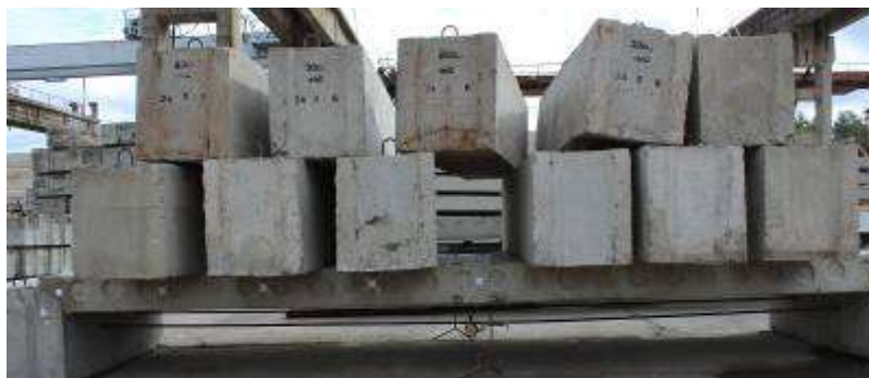
Figure 7 – Experimental sample of inter-column slab with pre-stressed working fittings during in-test
