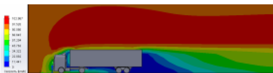
Figure 17 – Flow chart of the main train with a low cabin and ordinary ramp
