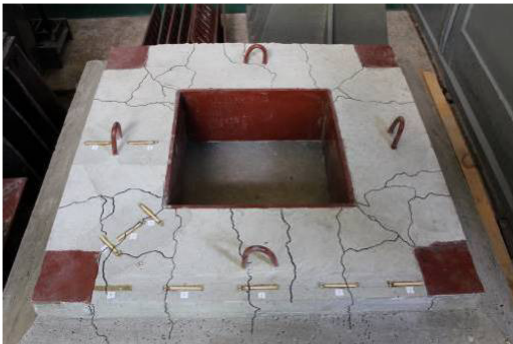
Figure 14 – Cracks in the concrete surface of a sample of PNA series
