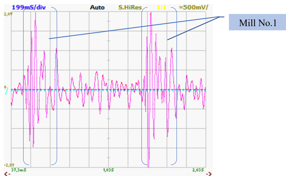
Figure 2 – Oscillogram of vibrations. Point No.1 Piliger mill No.1 is in operation. (1 div. Y axis = 3.75 \mu\text{m} , 1 div. X axis = 0.2 s)
