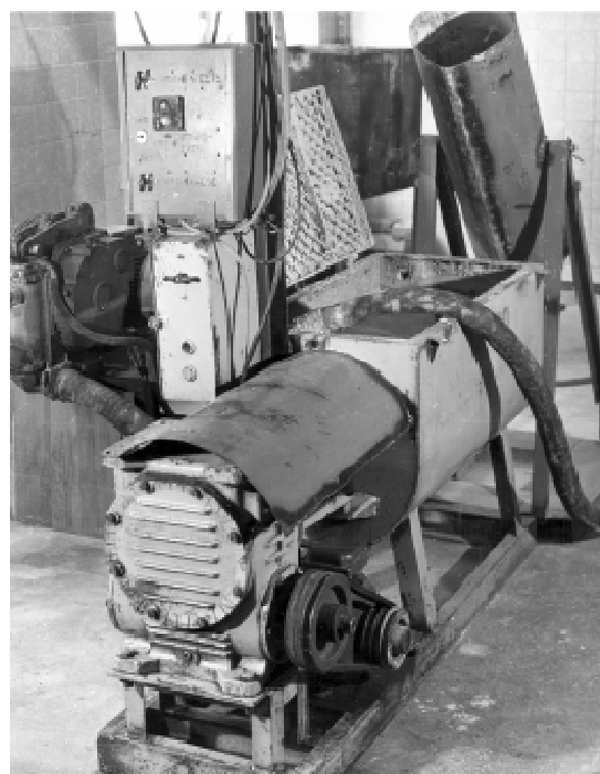
Figure 3 – Experimental installation for grout pumps study
