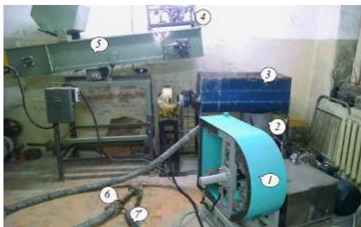
Figure 2 – Small-sized technological set equipment for carrying out a gunite work by wet method:
