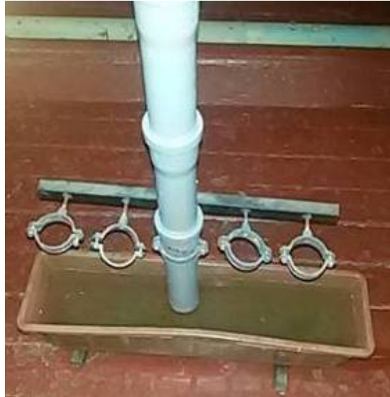
Figure 1 – Chute, filled with water for possible capillary ascension research for road embankment
