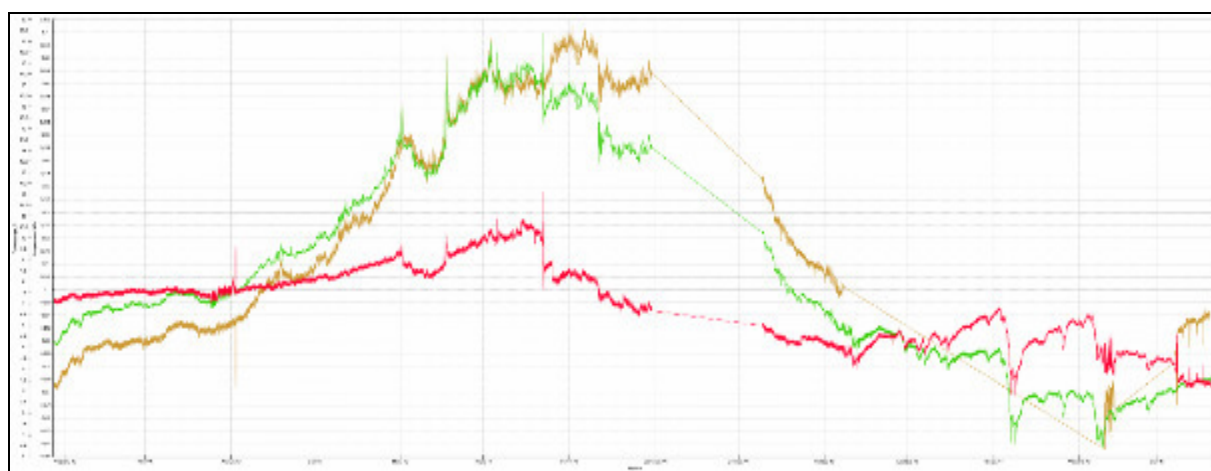
Figure 6 – Graph of changes in temperature and stresses occurring in pillar structures from December 2015 to March 2017
