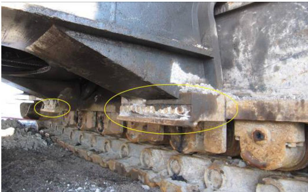
**Figure 2 – The location of the supporting platforms on the traverse of the excavator**
