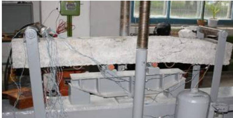
**Figure 9 – Investigation of beam 1B – FC – 1 on flexure**
