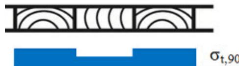
**Figure 9 – Uneven distribution of stresses by tension perpendicular to grain**
