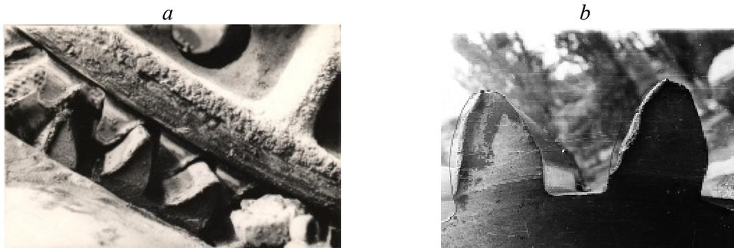
**Figure 2 – Profiles of the open gear wheels gear during their long-term operation:**
