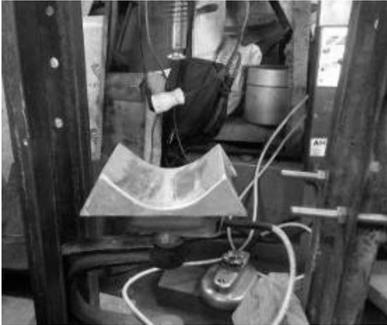
**Figure 1 – The new reinforced vulcanizer frame**
