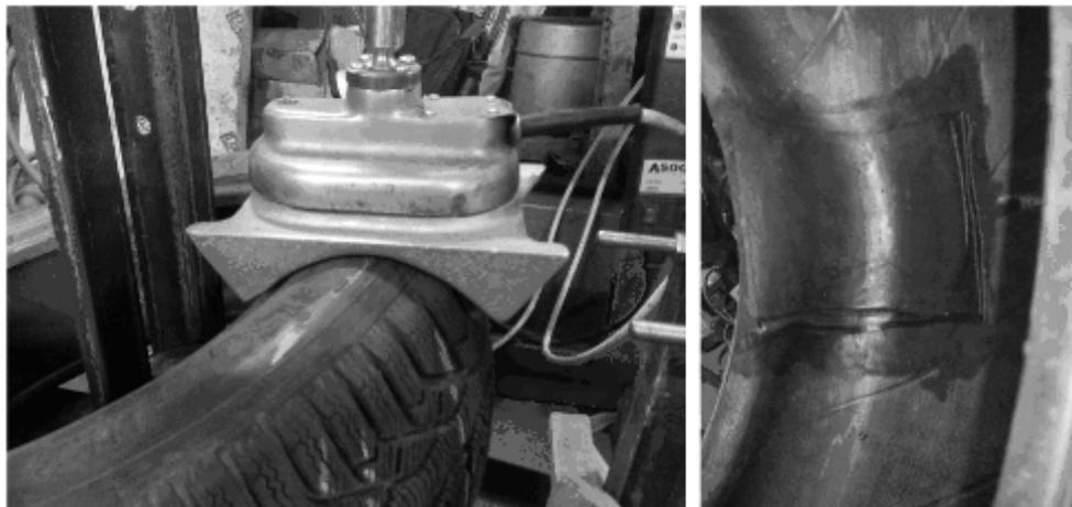
**Figure 6 – The control automobile tire vulcanization**
