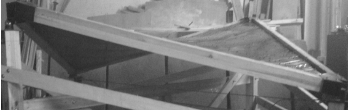
Figure 5 – Side view of the shell from a parabolic panel size 3 \times 3 \times 0,35 m in the laboratory of the department MW&PC, OSABA.
