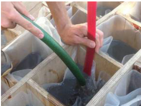
Figure 13 – Adjusting a water level in cells
