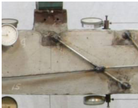
Figure 2 – Starting position of the inclined bar at an angle of 30^\circ , before load application.
