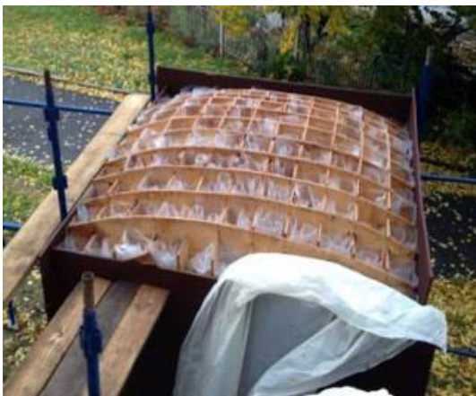
Figure 5 – A general view of the cell pool to test the spherical shell
