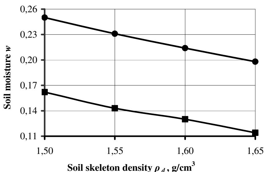
**Figure 2 – Plots relation of soil moisture  $w$  at what the light loam was compacted from soil skeleton density  $\rho_d$  (curve with domed markers), and final average soil moisture  $w_k$  of already compacted light loam from  $\rho_d$  within tube height (curve with squarely markers)**
