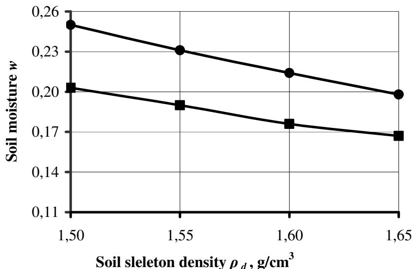
**Figure 1 – Plots relation of soil moisture  $w$  at what the heavy loam was compacted from soil skeleton density  $\rho_d$  (curve with domed markers), and final average soil moisture  $w_k$  of already compacted heavy loam from  $\rho_d$  within tube height (curve with squarely markers)**
