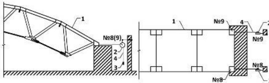
**Figure 7 – Placement of instruments for measuring displacement of support nodes:**
