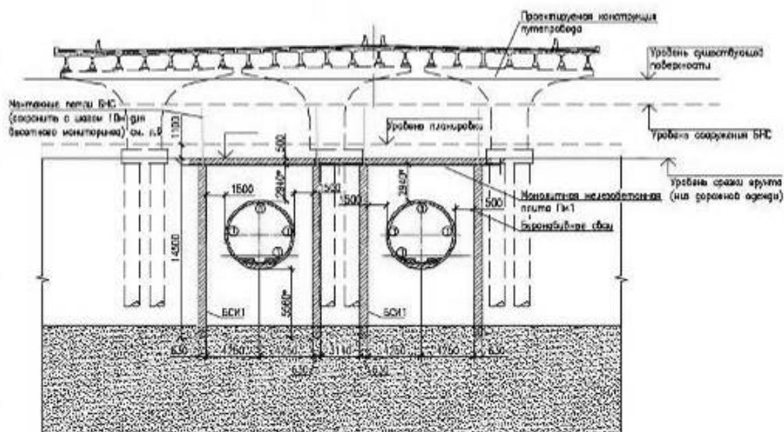
**Figure 2 – Cross section of a multilevel transport interchange**
