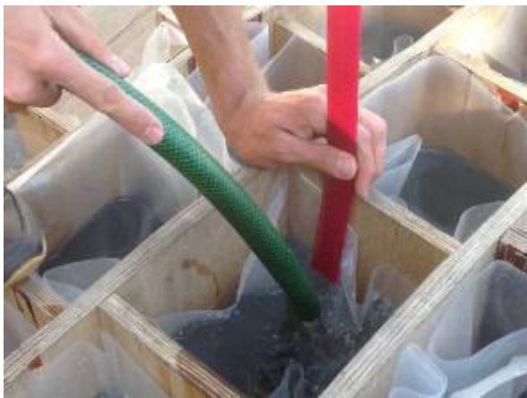
Figure 13 – Adjusting a water level in cells
