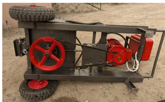
Figure 3 – Placement of pulleys on the engine and working body
