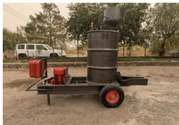
Figure 1 – Installations for the preparation of aerated concrete
