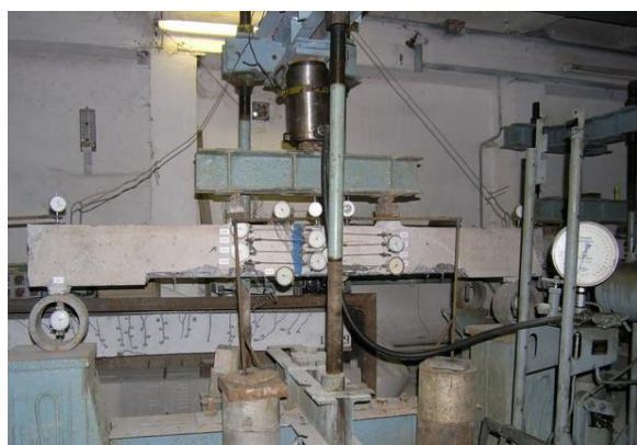
Figure 1 – The appearance of reinforced concrete beams from series 2 and beams from series 3, which were strengthened under load by welding directly to the existing longitudinal reinforcement or to short reinforcement segments (short bars) (top photo), tested in study [2] by researcher Ya. Rymar.
