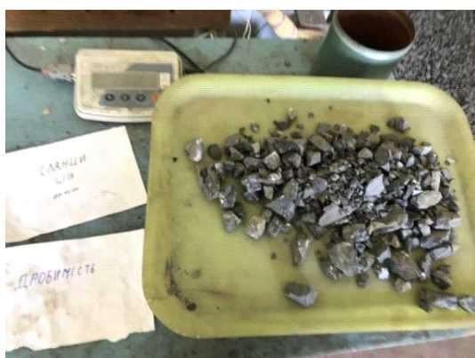
Figure 6 – Weighing of crushed stone sample from schists after loading (Source: Author’s photo)
