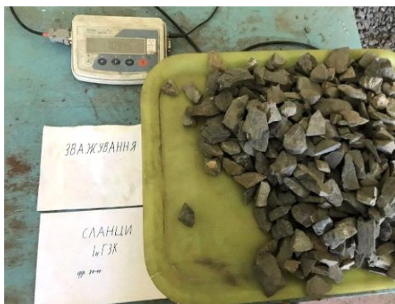
Figure 3 – Weighing of the 20–40 mm crushed stone fraction from schists on electronic bench scales ” (Source: Author’s photo)
