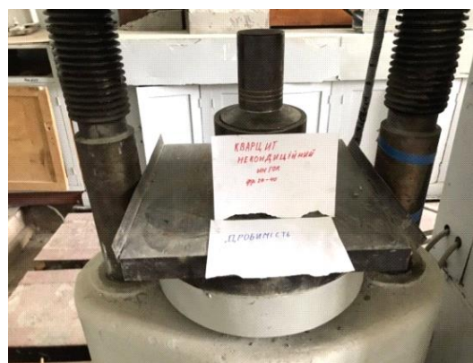
Figure 5 – Crushed stone sample from substandard quartzites in the cylinder under the plunger before loading (Source: Author’s photo)
