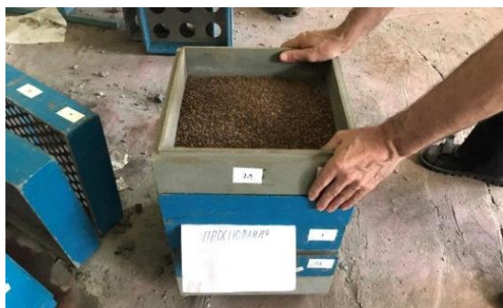
Figure 2 – Sieving of 5–70 mm fraction from oxidized jaspilites, PJSC “InGZK” (Source: Author’s photo)
