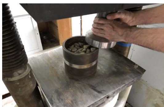
Figure 4 – Filling the cylinder with migmatite crushed stone before testing (Source: Author’s photo)
