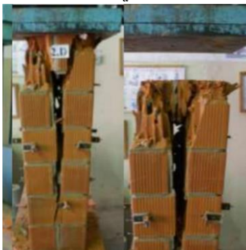
Figure 6 – The nature of the destruction of masonry columns under compression according to: a – [4]; b – [1]
