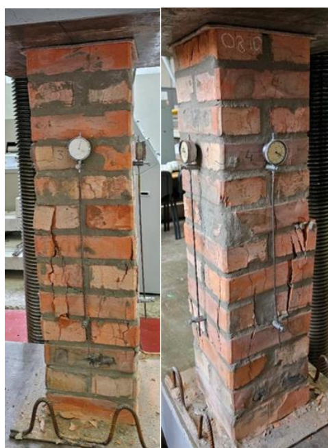
Figure 3 – Masonry test column C-25.25.100 after testing
