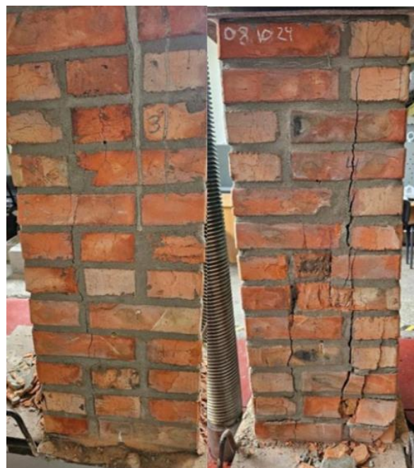
Figure 4 – Masonry test column C-38.38.100 after testing
