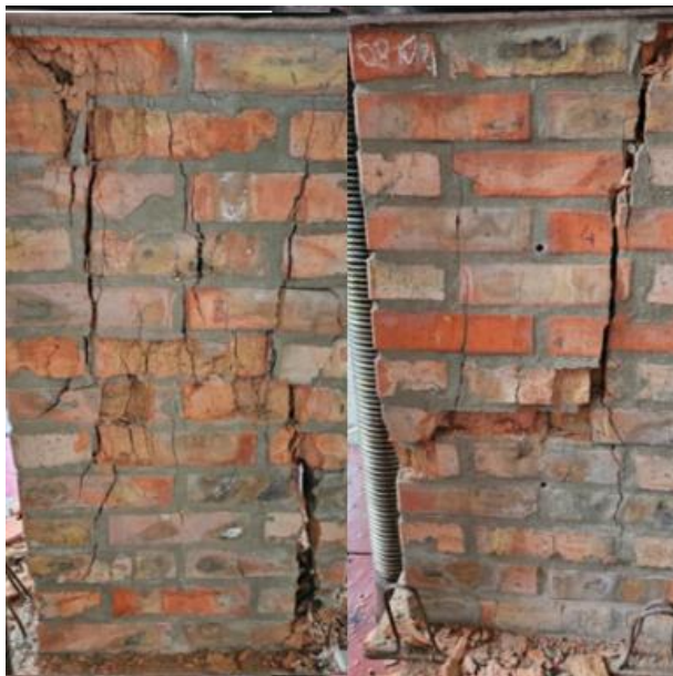
Figure 5 – Masonry test column C-51.51.100 after testing
