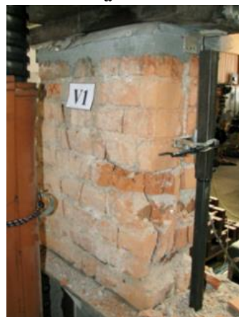
Figure 8 – The nature of wall destruction under axial compression in laboratory tests: a – [6, 7]; b – [6]
