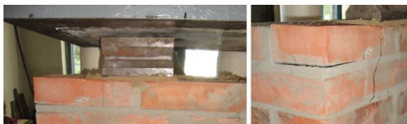
Figure 23 – Test sample W-2-15×10: a – during testing; b – nature of destruction
