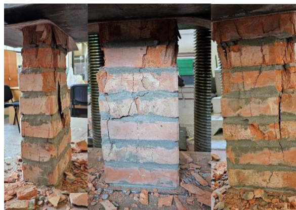
Figure 13 – Test sample P-25.12.51.5-a after testing
