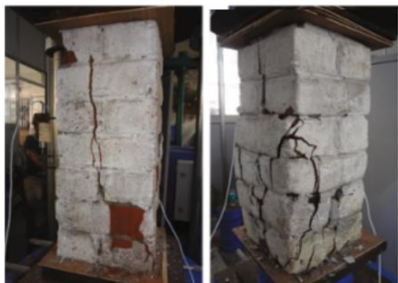
Figure 5 – Masonry test column C-51.51.100 after testing
