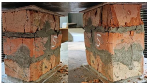
Figure 9 – Test sample P-25.12.21.5-a after testing
