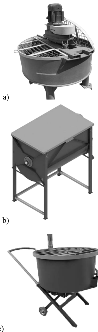
Figure 1 - Forced-action concrete mixers, a) RSP-800, b) SGSh-500, c) BP2-100.
