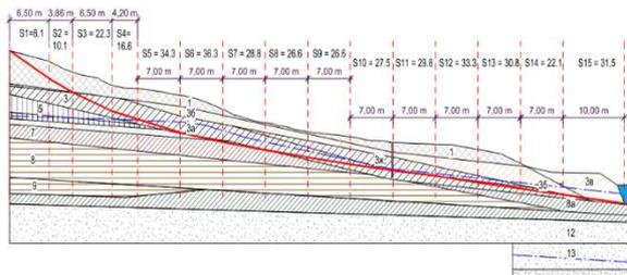
Figure 15 – Calculation scheme of slope stability
