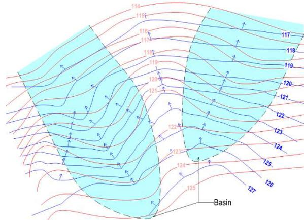
**Figure 8 – The scheme of placing basins on the slope**
