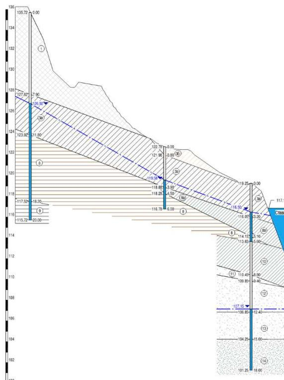
**Figure 4 – Longitudinal engineering geological section**
