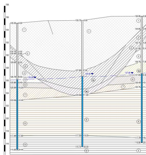
**Figure 5 – Transverse engineering and geological section**
