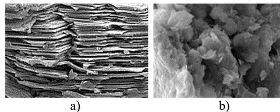
**Figure 9 – The structure of clays (a) and loess loams (b)**
