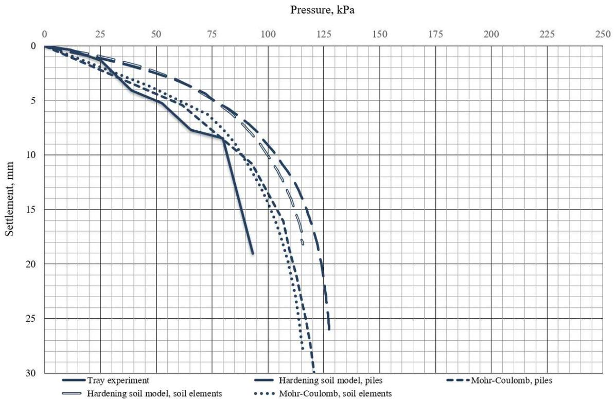
**Figure 4 – Results of the tray experiment and the FEM numerical modeling in 3D setting of stamp tests of unreinforced soil base in a tray**
