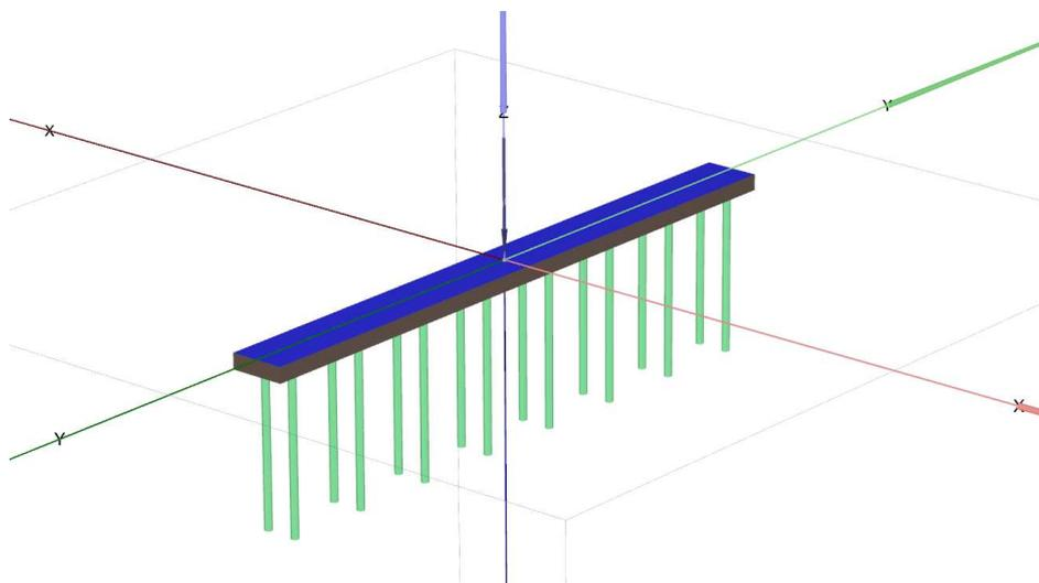
**Figure 1 – Soil-cement elements formed by volumetric soil elements**
