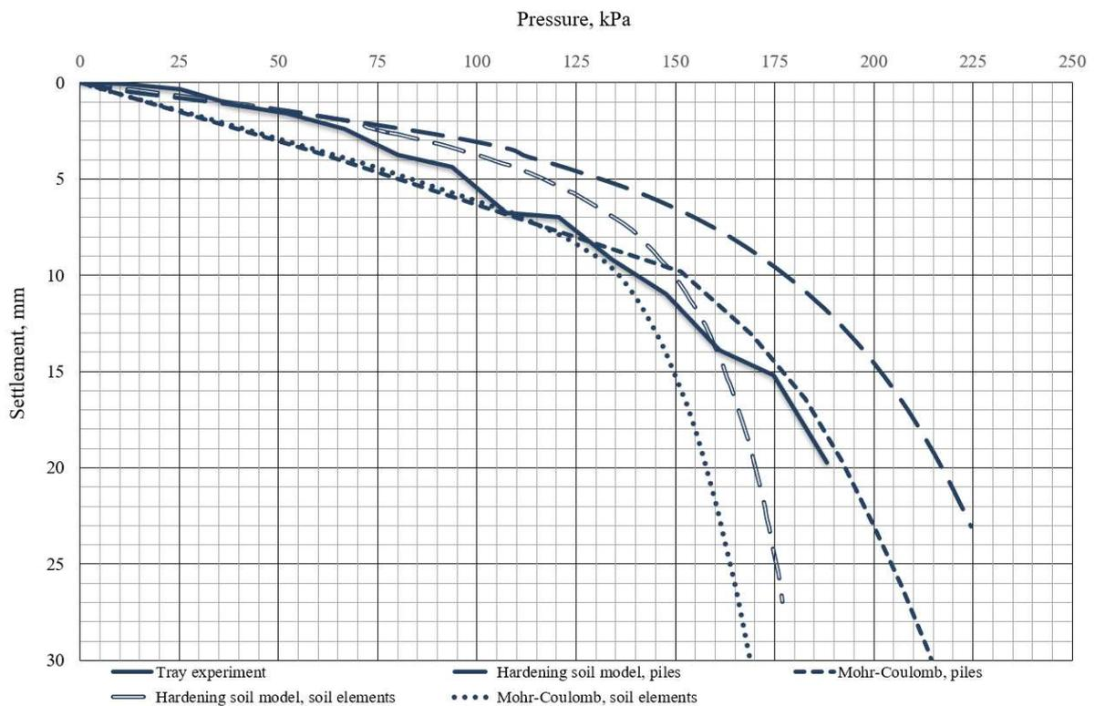
**Figure 6 – Results of the tray experiment and the FEM numerical modeling in 3D setting of stamp tests of soil base in a tray with a reinforcement percentage of 4.4%**
