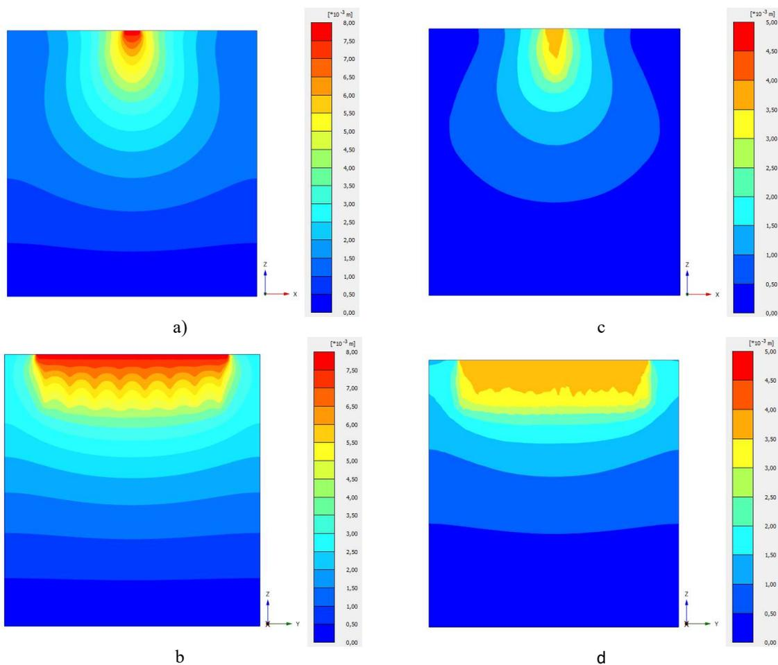
Figure 3 – Settlements of soil base with reinforcement percentage of 2,1% under a load of 1,5 kPa:
