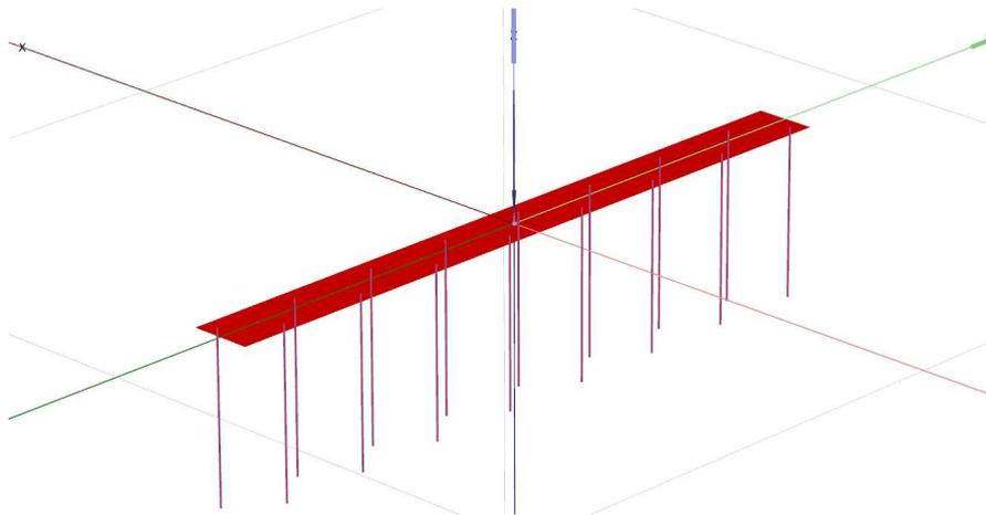
Figure 2 – Soil-cement elements formed by pile elements “embedded beam”
