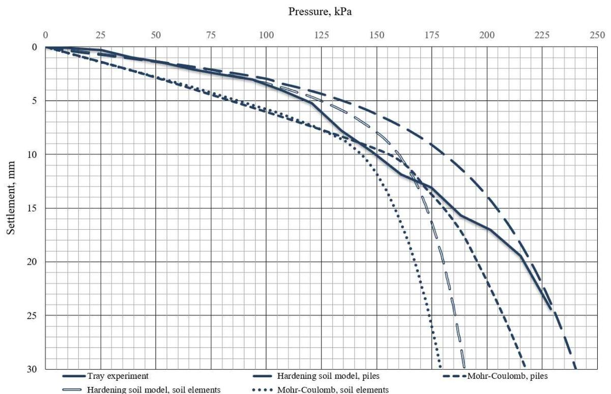
**Figure 7 – Results of the tray experiment and the FEM numerical modeling in 3D setting of stamp tests of soil base in a tray with a reinforcement percentage of 7.1%**
