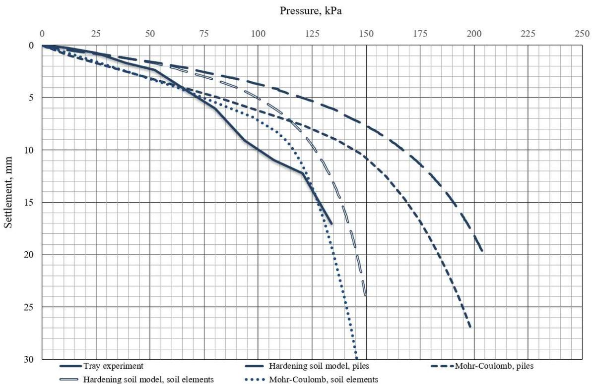
**Figure 5 – Results of the tray experiment and the FEM numerical modeling in 3D setting of stamp tests of soil base in a tray with a reinforcement percentage of 2.1%**
