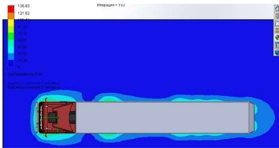
**Figure 12 – Diagram of air vorticity distribution around a road train at a speed of 100 km/h with a fairing of the lower part of the trailer and a Henning-Marxen bag tail**
