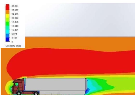
**Figure 11 – Diagram of wind speed distribution around a road train at a speed of 100 km/h with a fairing of the lower part of the trailer and a Henning-Marxen bag tail and an rear wing**
