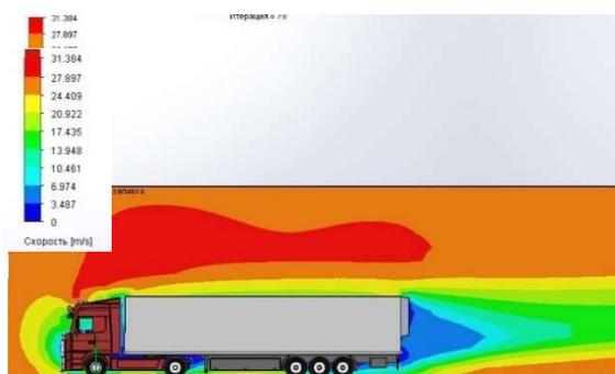
**Figure 9 – Diagram of air speed distribution around the road train at a speed of 100 km/h with a wing-skirt located behind**
