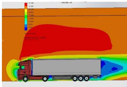
Figure 3 – Diagram of air speed distribution around the road train at a speed of 100 km/h
