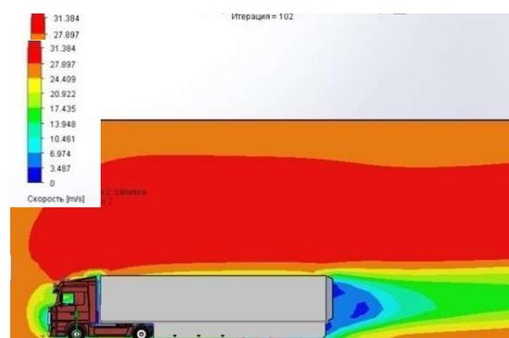
**Figure 10 – Diagram of the air velocity distribution around the road train at a speed of 100 km/h with the fairing of the lower part of the trailer and the tail of the Henning-Marxen bag**
