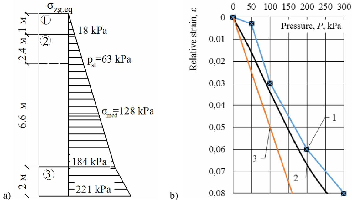
**Picture 6 – Calculation of soil collapsible deformations from its own weight:**
