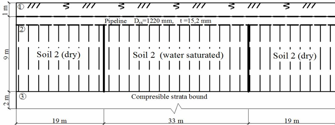
**Picture 5 – Pipeline in the loessial soil with collapsible property (central area in the water saturated state, side areas in the natural condition)**
