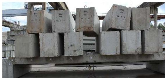
**Figure 10 – Test sample of inter-column slab during testing**
