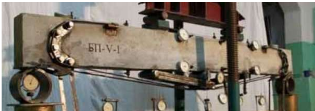
Figure 3 – General view of the reinforced concrete beam reinforced by the rod-roll system during the test
