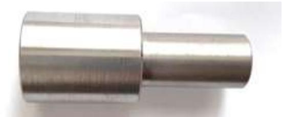
**Figure 5 – Plunger with an important diameter of 30 mm**
