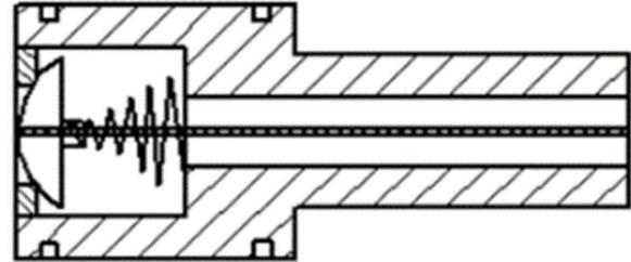
Figure 13 – Plunger made of steel (split)
