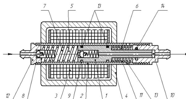
**Figure 1 – Differential pump of electromagnetic action:**
