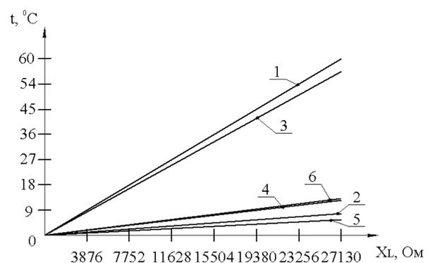
**Figure 17 – Graph of the dependence of the heating temperature of the plunger on the winding resistance:**
