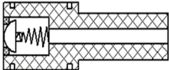
Figure 14 – Plunger made of ground iron
