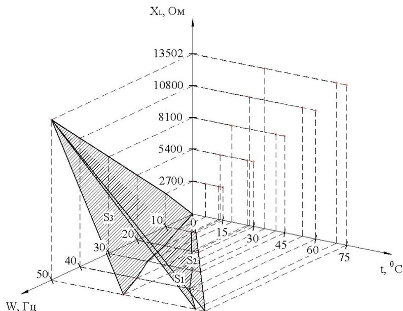
**Figure 18 – Three-dimensional graph of temperature-resistance characteristics**
