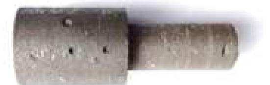
**Figure 8 – Plunger with a thickness of 30 mm**
