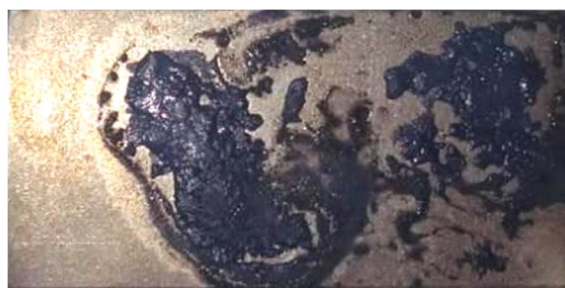
Figure 3 – Sample after prolonged exposure to ultrasound
