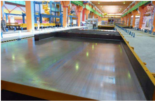
Figure 10 – Molding pallet for the production of panels
