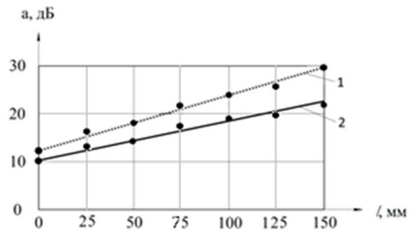
**Figure 6 – Value change graph of shock pulses  $a$  (dB) depending on the lever length, fixturing the vibration exciter  $l$  (mm), relationships ratio: 1 - theoretical, 2 - experimental**
