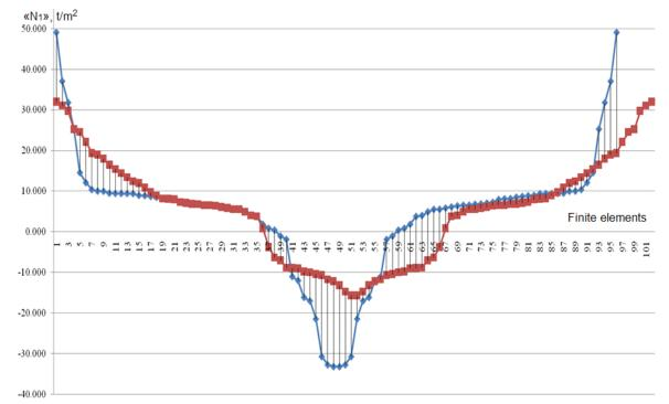
Figure 7 – Diagrams the major stresses «N₁» with symmetrically loading domes by snow load: → umbellate dome; → folded dome
