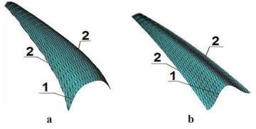
Figure 4 – Formation surface of the wave dome (the surface of the transfer): a – generatrix is a parabola; b – generatrix is sinusoid; 1 – curve generatrix; 2 – curves guiding
