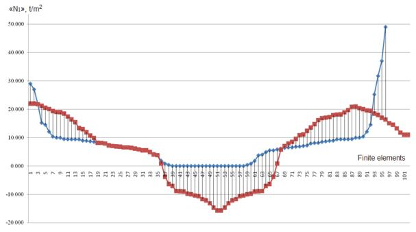
Figure 9 – Diagrams the major stresses «N<sub>1</sub>» with unsymmetrical loading domes by snow load: ---- umbellate dome; ----- folded dome
