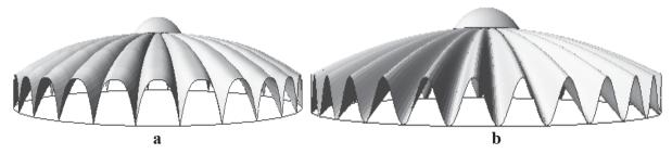
Figure 3 – The calculation schemes of wavy concrete domes: a- umbellate dome; b- folded dome
