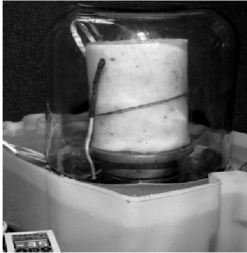
**Figure 3 – A device for studying the melting of process of gas hydrates**
