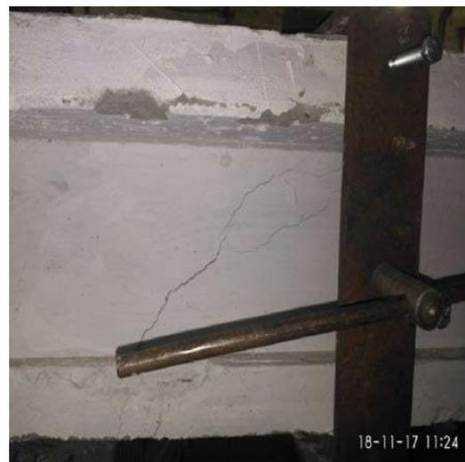
**Figure 11 – General view of of an inclined crack at the edge**
