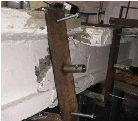
**Figure 7 – The destruction of the beam**
