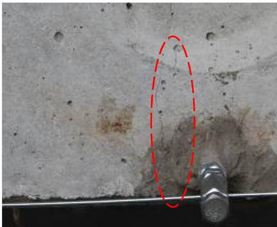
**Figure 9 – Occurrence of the first cracks near the average cross section at a total load of 163 kN, such as pre-stressed PNC**
