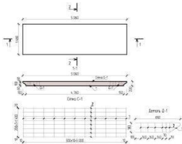
**Figure 5 – Reinforcing frame and PMC parts**
