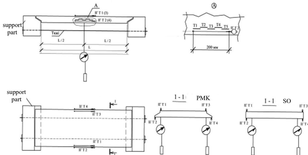
Figure 3 – Arrangement of measuring devices on the intercolumn plate
