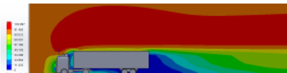
Figure 20 – Flow chart of the main train with a with a low cab and located behind the improved ramp
