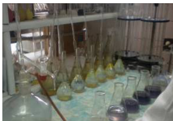
Figure 2 – Titration of the water samples taken to determine the content of iodine
