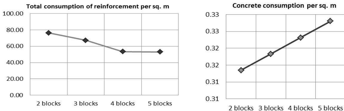
**Fig. 16. Total consumption of reinforcement per 1 sq. m.**
