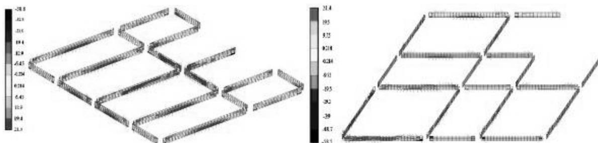
**Fig. 20. Crack distribution in beams adjacent to the damaged cells**
