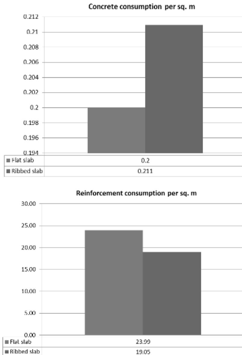
**Fig. 21. Consumption of concrete m<sup>3</sup>/m<sup>2</sup> and reinforcement kg/m<sup>2</sup>**
