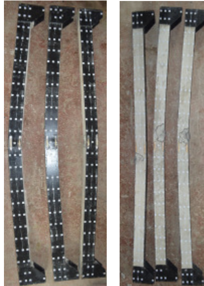
Figure 9 – The destruction of experimental steel-concrete samples with sheet reinforcement of the series SB-PD-24-1..3 and SB-PN-24-1..3 nature
