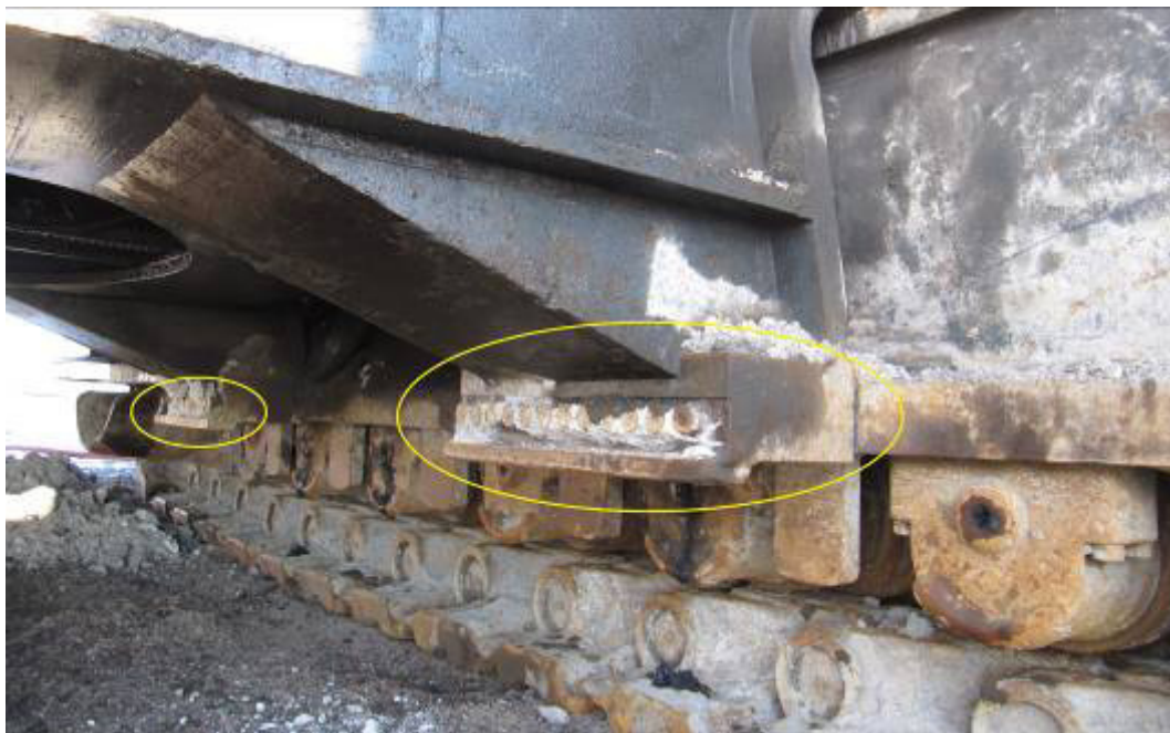
Figure 2 – The location of the supporting platforms on the traverse of the excavator
