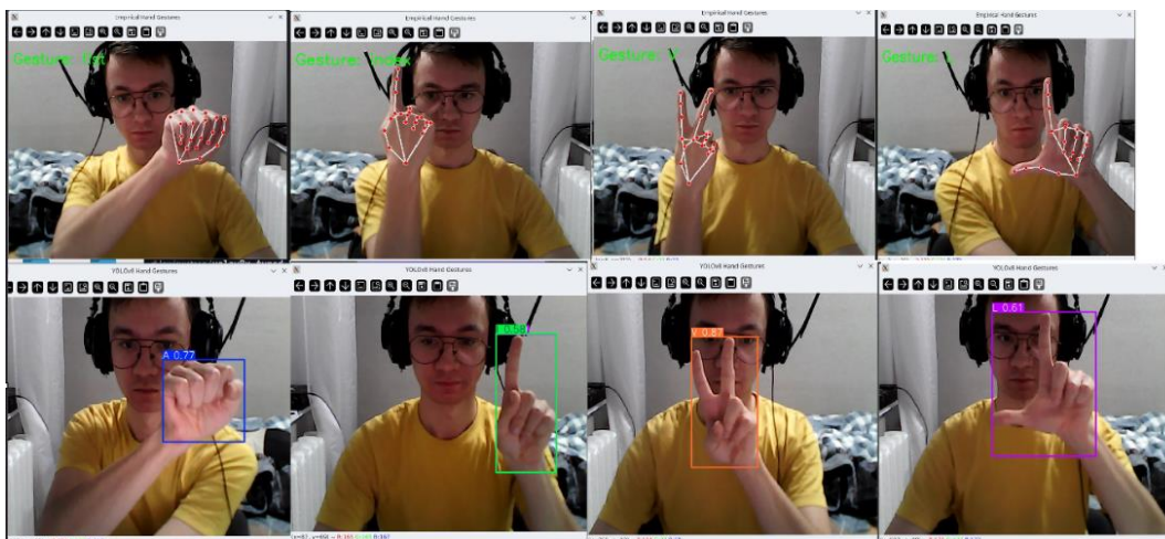
Fig. 7. Set of gestures recognised by the implemented systems based on MediaPipe Hands and YOLOv8 models
