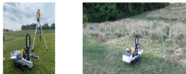
Fig. 1. Details of demining robot. On the left, is the robot with the on-board GPS system and off-board GPS tower; on the right, a panoramic view of the robotic platform scanning the test field
