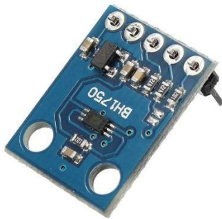
Fig. 3. Photodiode-based light sensors BH1750
