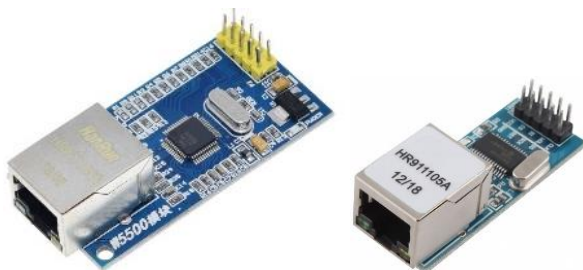
Fig. 5. WIZnet W5500 (on the left) and ENC28J60 (on the right)
