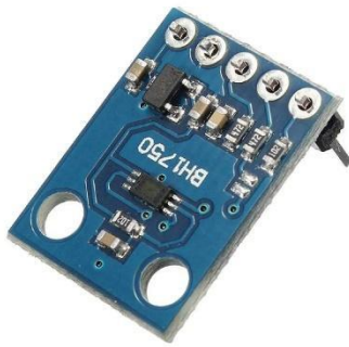
Fig. 3. Photodiode-based light sensors BH1750
