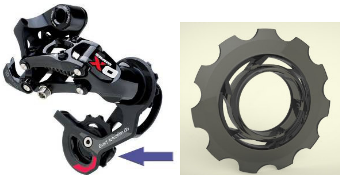
Figure 1 – Rear derailleur (left) and its idler lower pulley wheel (visualization)
