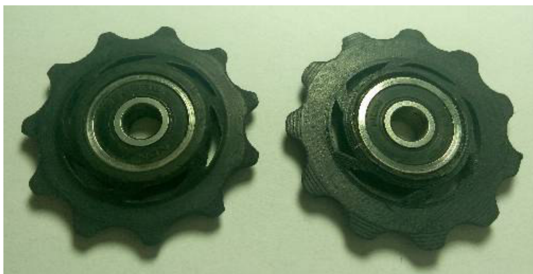
Figure 5 – Tooth gear wheel: the original (left) and the printed part
