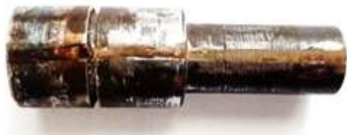
**Figure 4 – Working body with a diameter of 23 mm**
